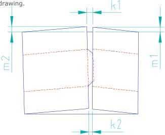
$\begin{array}{ll} \textbf{4.3.1.} & \text{Tilt} & \text{measure } m_1 \text{ and } m_2 < \text{thickness of corrugated board,} \\ & \text{still} < 5 \text{mm} \\ \textbf{4.3.2.} & \text{Gluing the "fishtail"} & \textbf{[k_1 - k_2]} < 1.5 \text{ thickness of corrugated board, still} \\ \end{array}$
