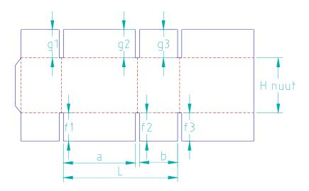
3.2 locations of openings (stripping ribbon, suspension openings, etc.)  $\pm$  3 mm
